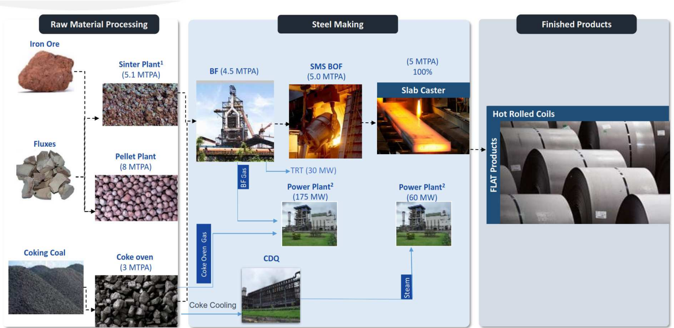
Fig 3 – Dolvi plant: Process flow in Phase-2 (5mtpa)
